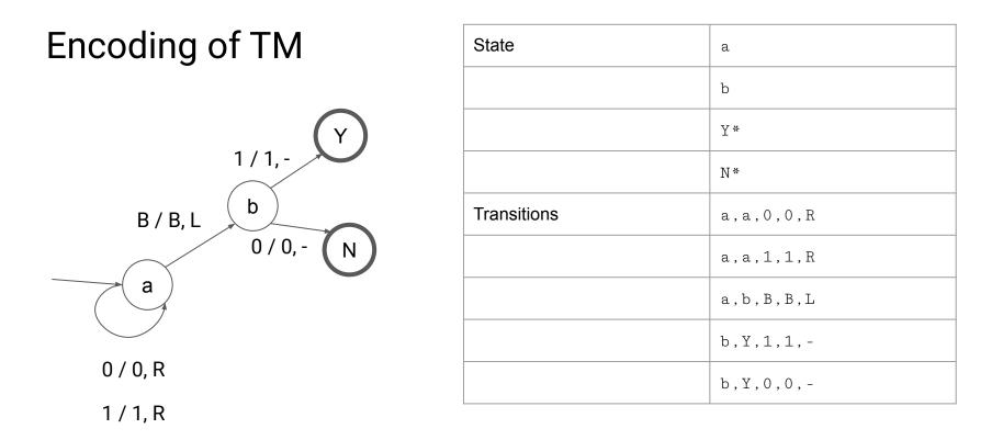
Encoding(M) = a, b, Y\*, N\*; a, a, 0, 0, R; a, a, 1, 1, R; a, b, B, B, L; b, Y, 1, 1, -; b, Y, 0, 0, -;
